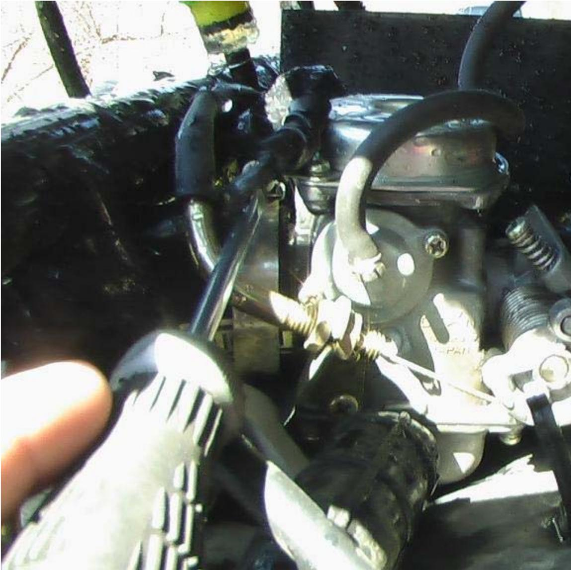
4) You may be able to tilt the carburetor to one side to reveal the bottom of the float bowl and the screws that keep it attached to the carb. Undrained gas may spill now. Some designs need carb removal or partial removal.
